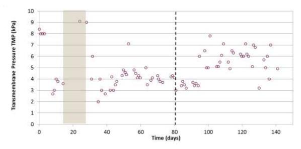
Figure 11: Transmembrane pressure in AnMBR pilot plant is stable indicates sustainable fouling.
