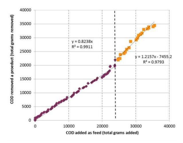
Figure 17: COD balance in the AnMBR pilot plant operated at 37°C. The slope of the linear regressions indicates the fraction of Feed COD that leaves the AnMBR as product (biogas and permeate).
