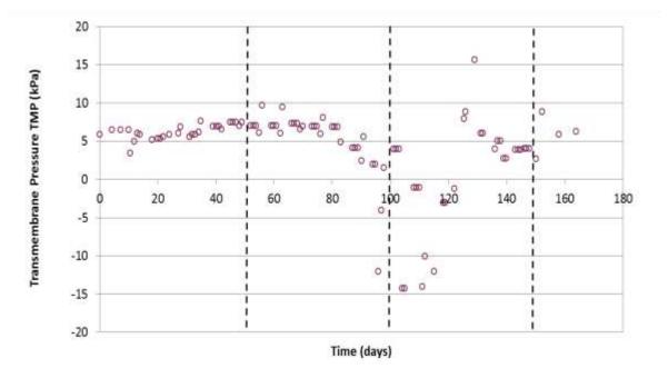
Figure 8: Transmembrane pressure in AnMBR pilot plant is stable indicates sustainable fouling.
