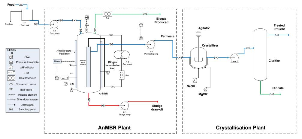
Figure 5: Detailed piping and instrument diagram of the integrated treatment process consisting of anaerobic membrane pilot plant and struvite pilot plant.
