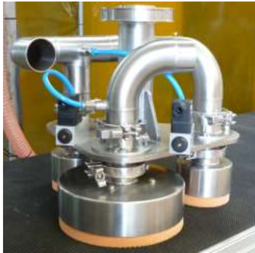
Fig. 12 Fabricated Gripper ready for mounting onto the robot
