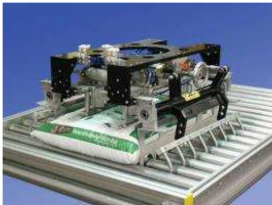
Fig 1. Mechanical and pneumatic grippers reviewed as possible options as part of the design process. The preference was for a pneumatic gripper as it was deemed that this would be the most suitable for picking up primals without causing damage to the vacuum sealed bag.
