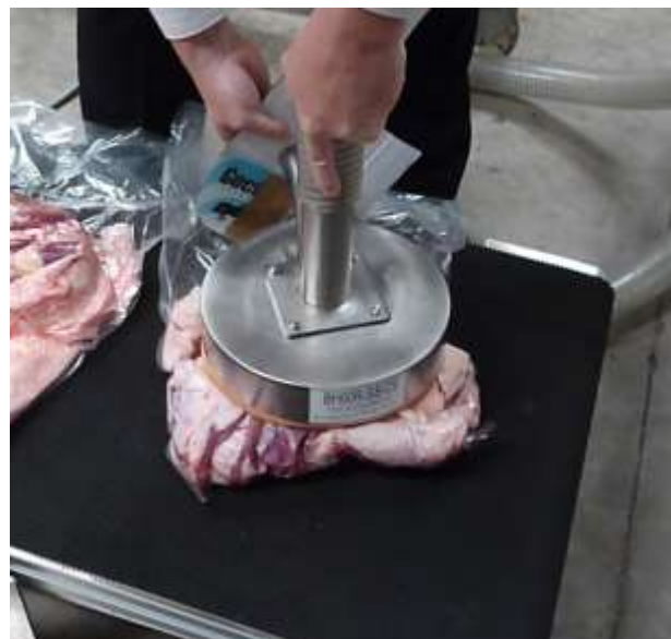
Fig.4 Trial gripper head picking up vacuum sealed primals in MAR's workshop - 1
