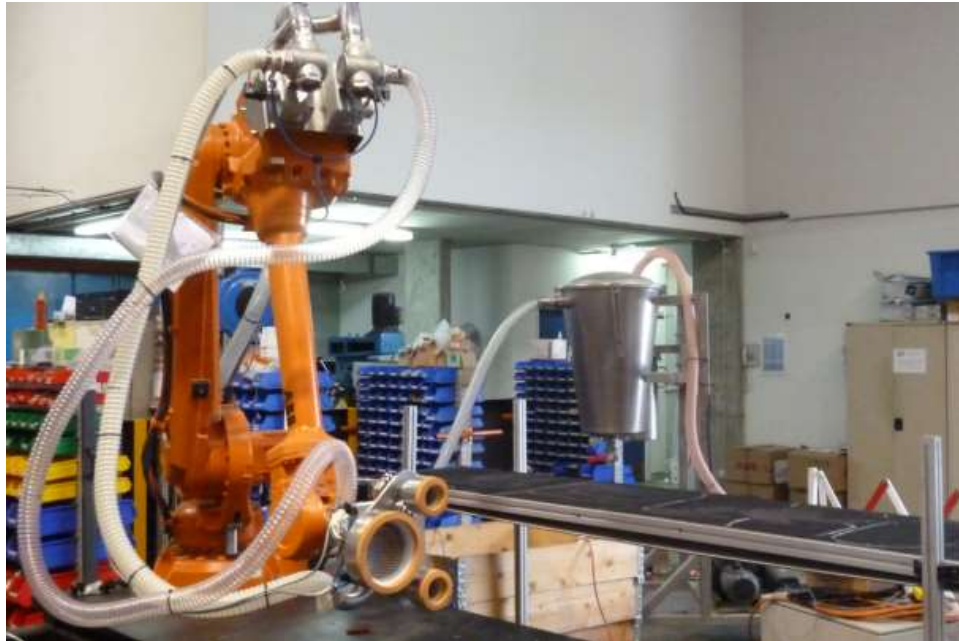
Fig. 13 The system setup for trials in MAR's workshop. The image shows the gripper, vacuum hosing and valving mounted on the robot, the vacuum system in the background with product conveyor in the middle.
