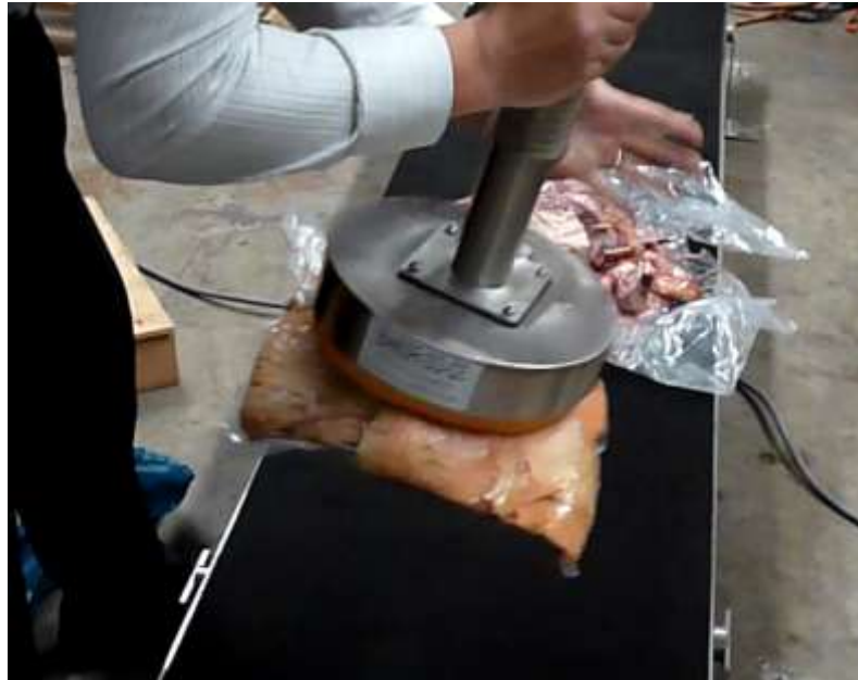
Fig.5 Trial gripper head picking up vacuum sealed primals in MAR's workshop - 2
