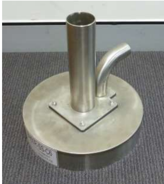
Fig.3 A trial Vacuum Gripper head was sourced and fabricated first before detailed design was conducted
