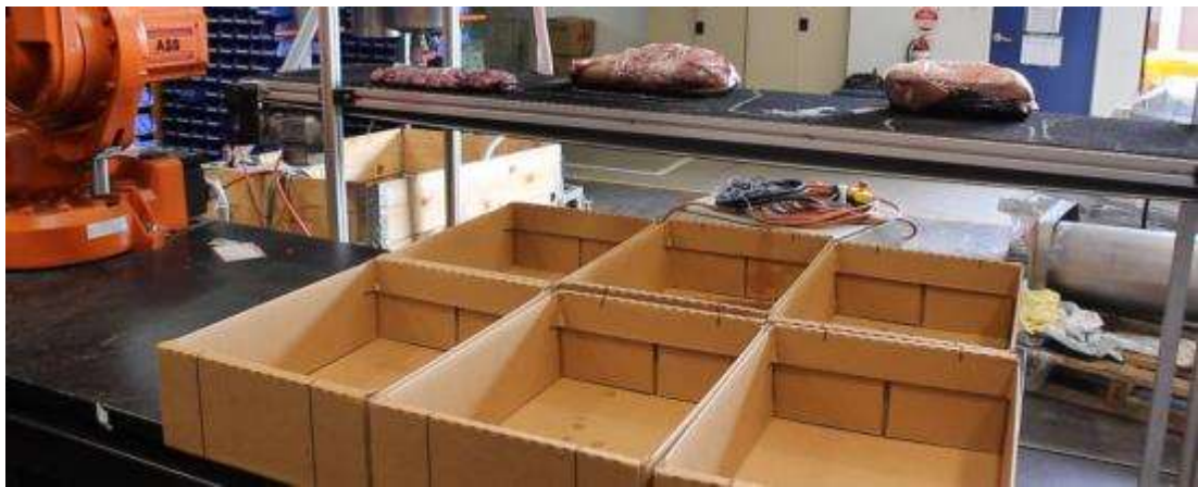
Figure 155: Image of cartons and robot on the robot base with the primals on the conveyor ready for pick up.
