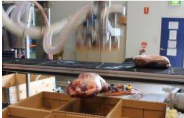
Figure 177: A large primal being dropped after place operation. This highlighted the need for pressure switches to ensure suitable vacuum had been lost before certain robot moves were initiated.
