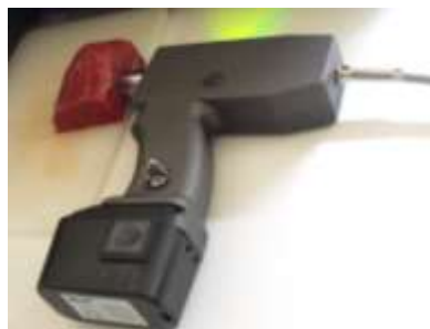
Figure 2. Hand held Raman spectroscopic device showing the measurement of the m. semimembranosus with the epimysium removed.
