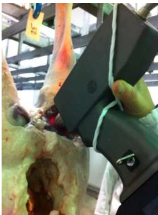
Figure 5. Pre- rigor measurement of the m. semimembranosus in-situ in processing plant conditions.
