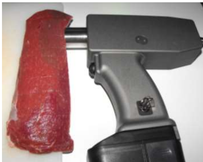
Figure 11. Hand held Raman Spectroscopy sensor head measuring the cranial portion of a fresh intact lamb LL with the epimysium removed, perpendicular to the muscle fibres.
