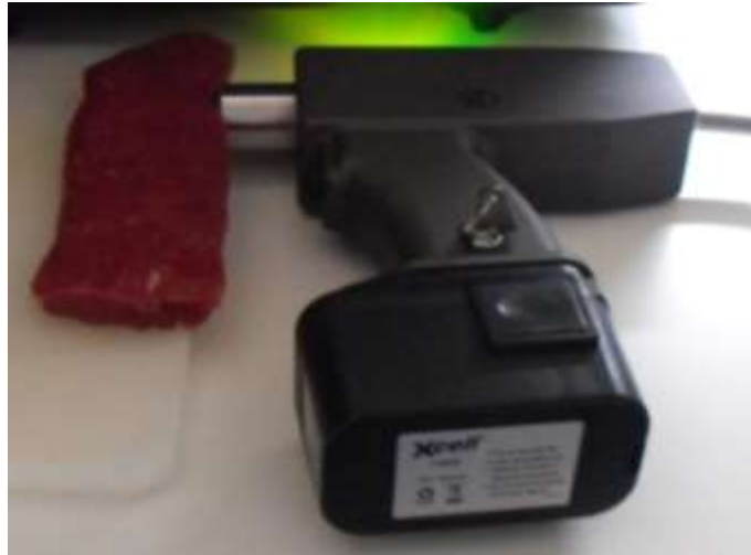
Figure 1. Hand held Raman spectroscopic device showing the measurement of the m. longissimus lumborum with the epimysium removed.
