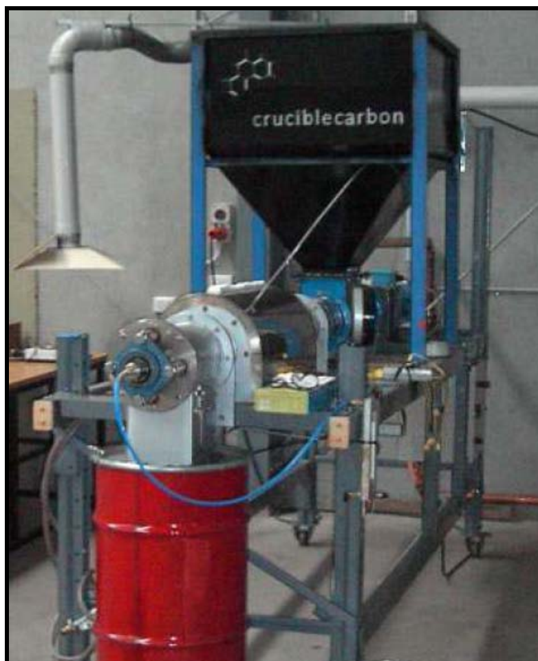
Figure 4.18: Picture of Crucible Carbon Pyrolysis Pilot Plant
