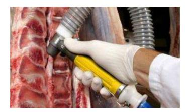
Fig. 2 The image shows one of the tools that is currently used manually to remove the spinal cord from beef sides. It consists of a circular rotating cutting blade that gets in behind the spinal cord and cuts the Dorsal Root Ganglia before vacuuming away the removed material.
