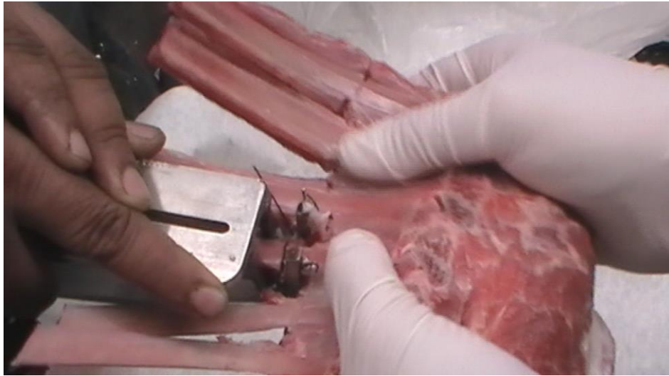
Figure 5: Rib clamped in U holders
