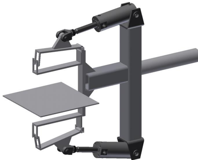
Figure 5. Twin-headed "U" Holder tool for meat desocking
