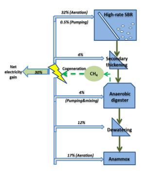
Figure 2: Flow scheme of potential electricity generation from the integrated high-rate wastewater treatment system.
