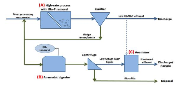
Figure 1: High-rate activated sludge process with integrated anaerobic digestion and anammox processes.
