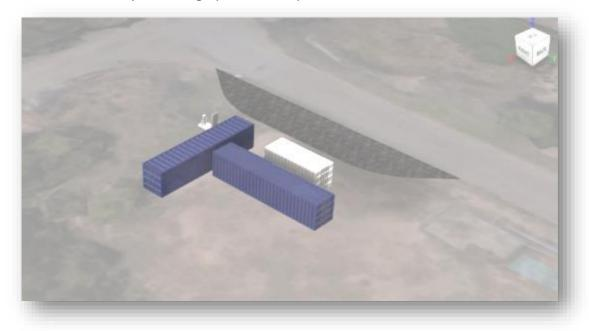
Figure 11: 1 MW electrolyser indicative Option 1 layout orthographic views.
