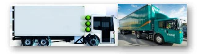
Figure 11: Econic refrigerated box option showing the H2 storage (green Fibre Reinforced Polymermer tanks or FRPs) and the Econic in a semi-trailer format.
