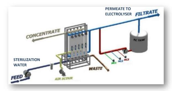
Figure 38: MAK Electrolyser Feedstock Water Pre-Treatment Schematic
