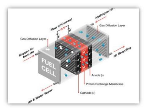
Figure 2: Schematic of a hydrogen fuel cell<sup>9</sup>.
