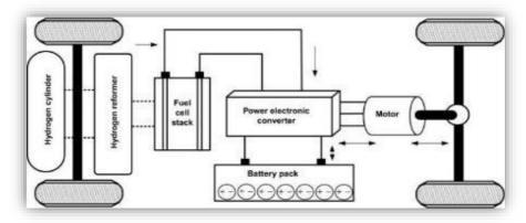
Figure 3: Schematic of a Fuel Cell-Electric Vehicle (FCEV) 10.
