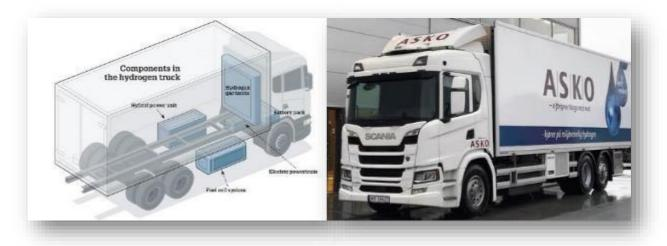
Figure 12: Scania H2 fuel cell truck.
