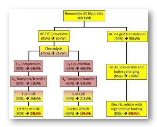
Figure 52: H2 and electric vehicle production routes, energy efficiency comparison
