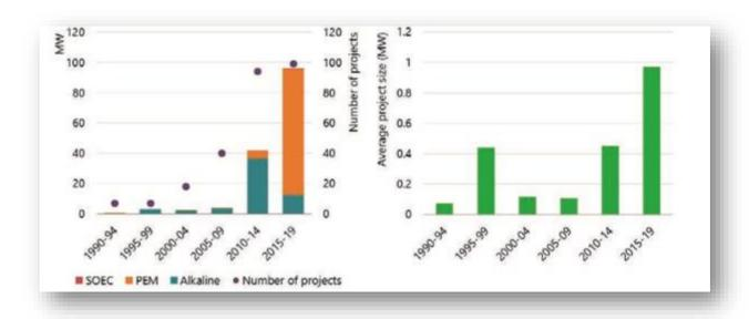
Figure 25: Development of electrolyser capacity for energy purposes and average unit size for the period 1990 to 2019.
