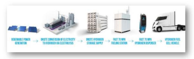
Figure 36: Example Ecosystem of H2 Transport System
