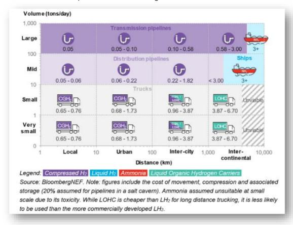
Figure 5: H2 transportation costs by volume and transport vehicle
