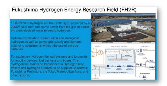
Figure 29: Case study of a recently commissioned 10 MW electrolyser in Japan.
