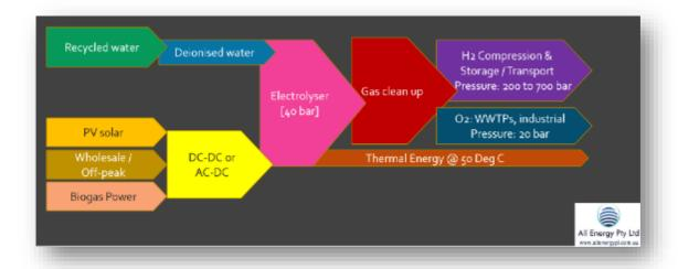
Figure 19: Block Flow Diagram showing production of renewable hydrogen via electrolysis.
