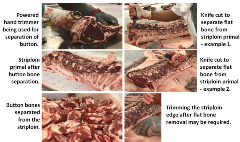
Figure 2: Current practice: removing button bones (left) and flat bones (right).
