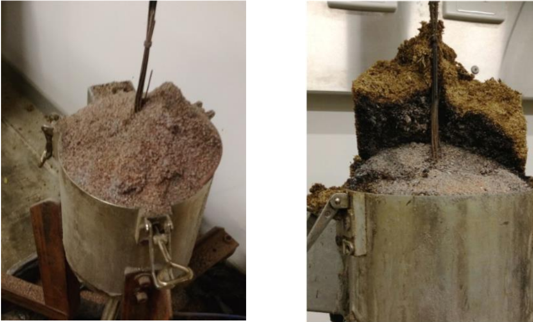
Figure 13: Ash and sand at the end of a self-sustaining experiment (left). Char and unburned waste at the end of a non-self-sustaining experiment (right)
