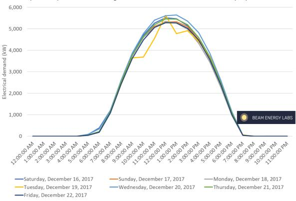
Figure 5: 7,000kWe solar PV generation profile during site peak demand, source: data extracted from <u>Beam Energy Labs, commercial solar platform</u>.
