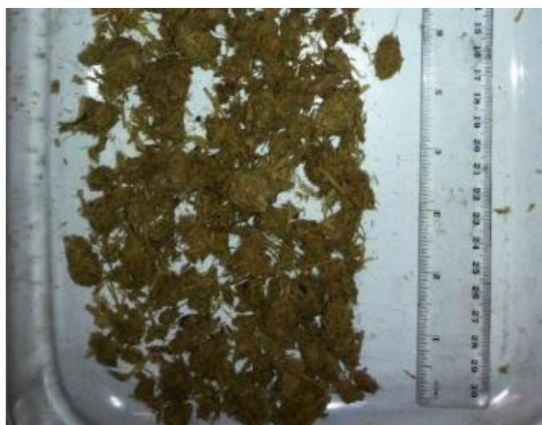
Figure 32: RMP5 Example of Screened and Dewatered Paunch Waste from RMP plant 2.
