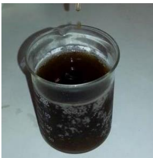
Figure 29: Sample of Beverage Waste to be used in co-digestion trials (FIO1). The waste has a very high soluble fraction with very small contribution to residual solids.
