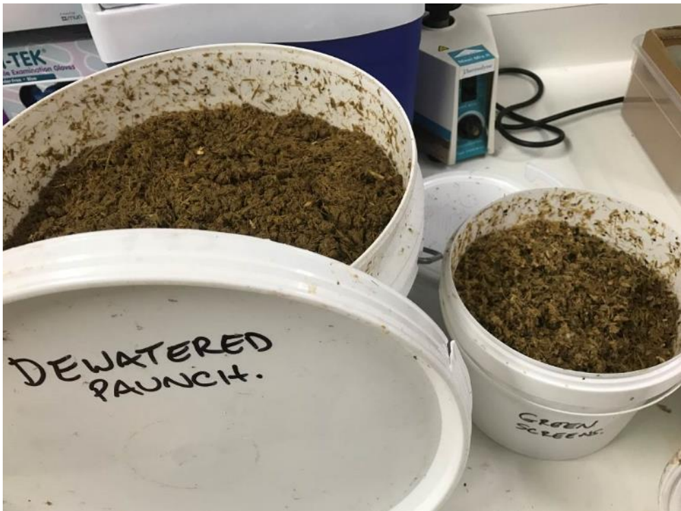
Figure 37 RMP1 – Example of Screened and Dewatered Paunch Solid Waste from RMP plant 1
