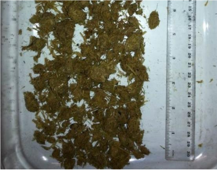
Figure 41: RMP5 Example of Screened and Dewatered Paunch Waste from RMP plant 2, supplied by QUU.
