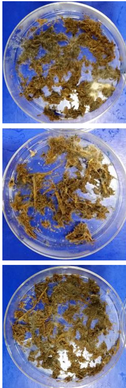
Figure 26 Solid state fermentation on raw solid paunch conducted using batch laboratory experiments inoculated with oyster mushrooms (top), anoki (middle) and aspergillus (bottom).
