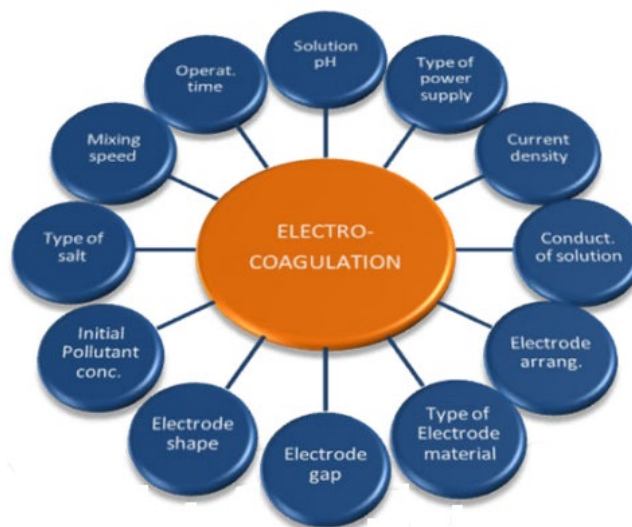
Figure 3: The many operating parameters influencing the EC process performance (Eyvaz, et al., 2014).
