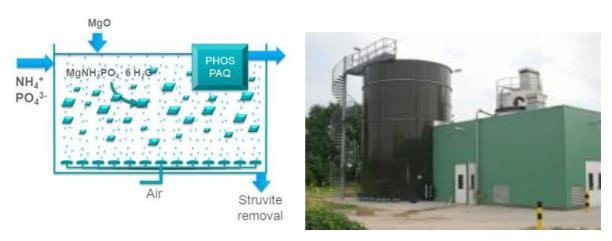
Figure 9: PhosPAQ Schematic
