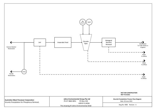
Figure 4: Process Flow Diagram specifying struvite crystallization placement in WWTP
