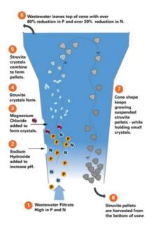
Figure 6: Multiform Harvest Process Schematic
