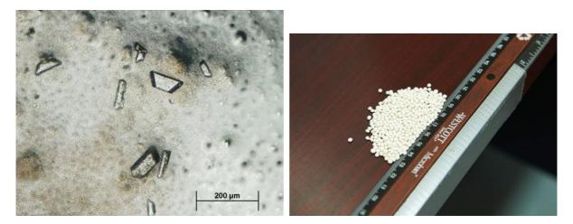
Photo 2: Individual Struvite Crystals
