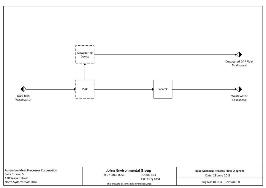
Figure 4. Base Case Scenario Process Flow Diagram
