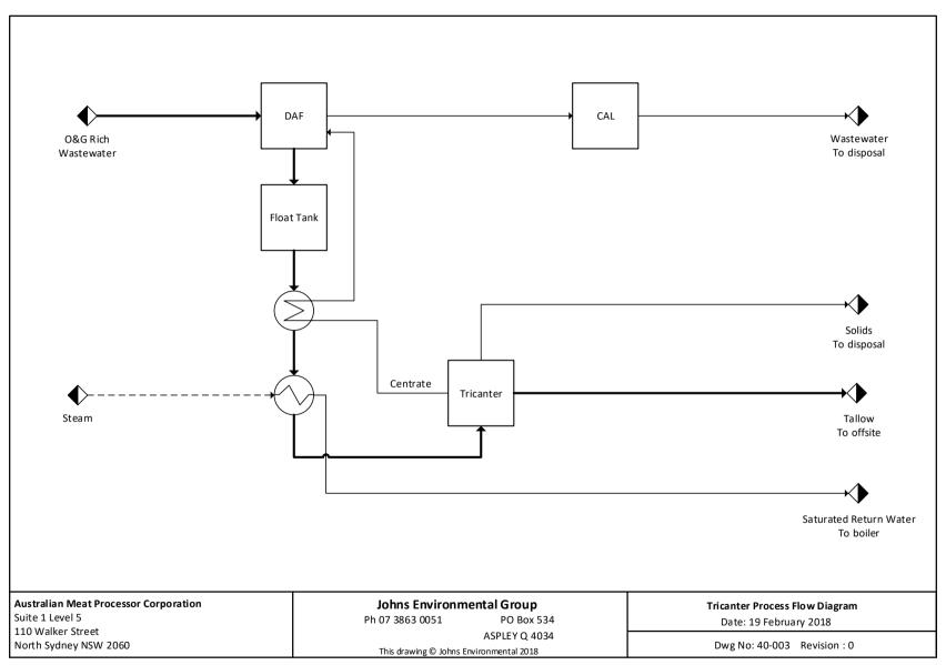
Figure 6. Tricanter Option (2) Process Flow Diagram
