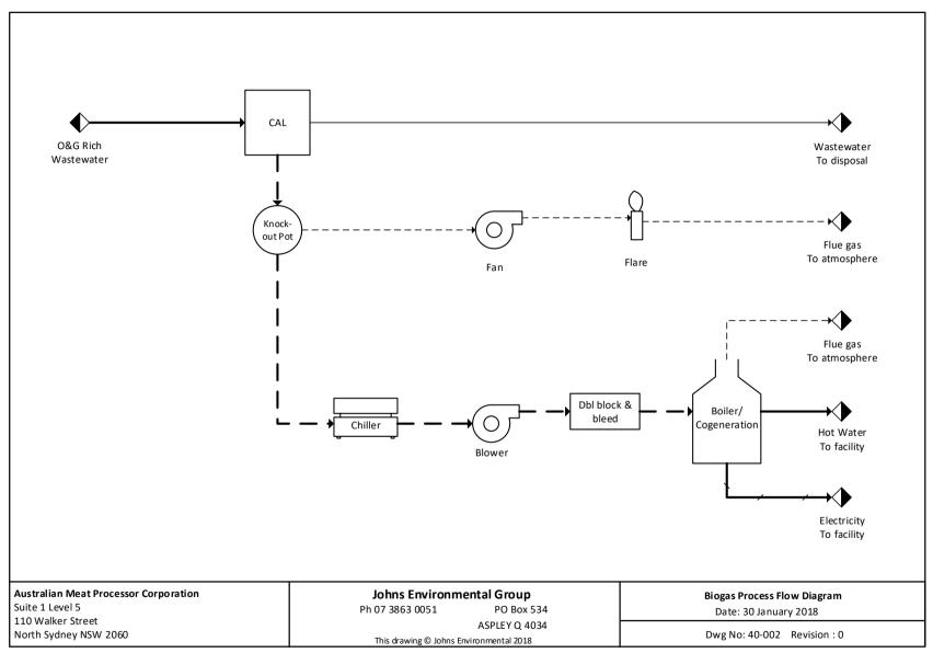
Figure 7. Biogas Option (3) Process Flow Diagram
