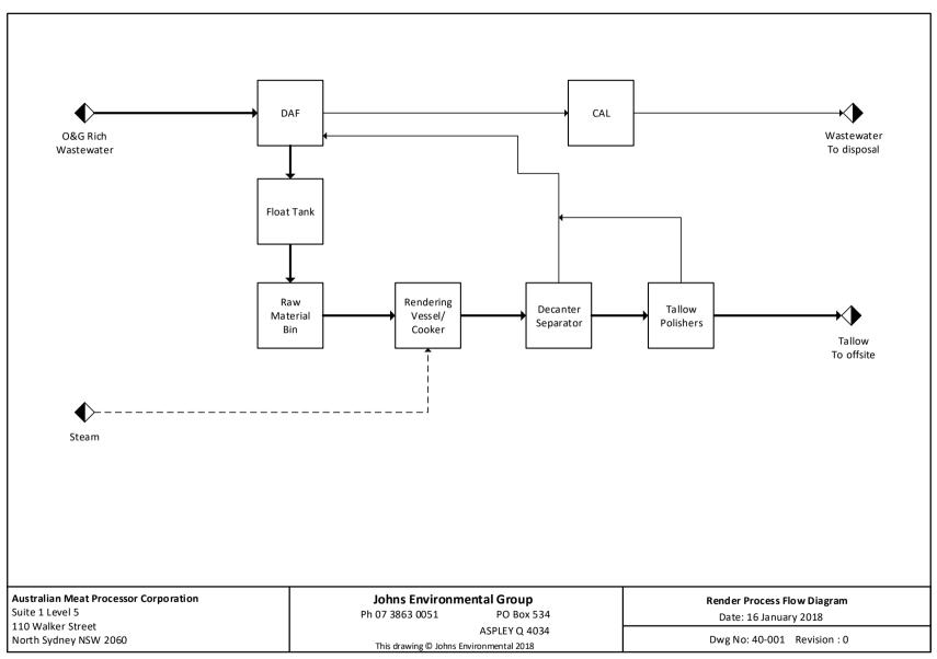
Figure 5. Render Option (1) Process Flow Diagram
