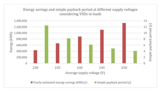
Figure 23: Annual energy savings and simple payback period when applying dynamic voltage optimisation (3 x 1 MVA and a 1.5 MVA unit) with a set voltage of 220V installed at a medium-sized abattoir with consideration of the effect of VSDs on the loads for a range of supply voltages
