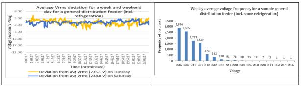
Figure 15: Deviation from the average V<sub>RMS</sub> on a week and weekend day for a transformer with a general distribution load (including some refrigeration) at a medium-sized abattoir Figure 16: Frequency of average line to neutral voltage over a week for a transformer with a general distribution load (including some refrigeration) at a medium-sized abattoir
