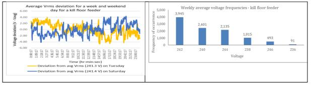
Figure 11: Deviation from the average V<sub>RMS</sub> on a week and weekend day for a transformer with a kill floor load at a medium-sized abattoir
