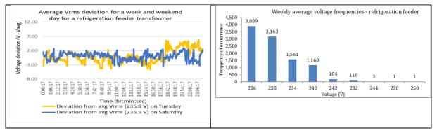
Figure 9: Deviation from the average VRMS on a week and weekend day for a transformer with a mostly refrigeration load at a medium-sized abattoir Figure 10: Frequency of average line to neutral voltage over a week for a transformer with a refrigeration load at a medium-sized abattoir
