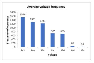
Figure 20: Average voltage frequency for a transformer connected to the main load
