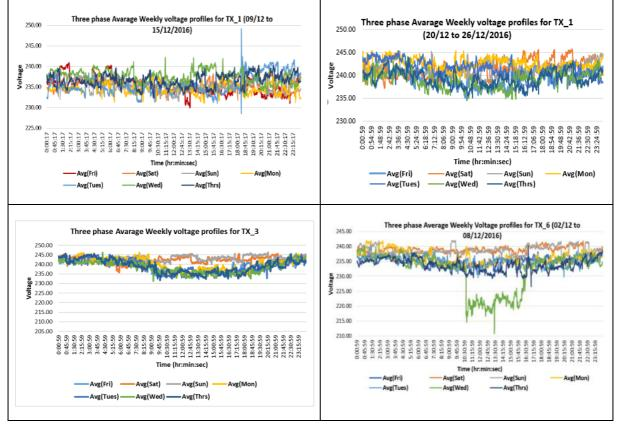
Figure 8 – Weekly average three -phase voltage profiles) for refrigeration (TX1), kill floor (TX2), by-products (TX3) and general distribution (TX6) feeder transformers
