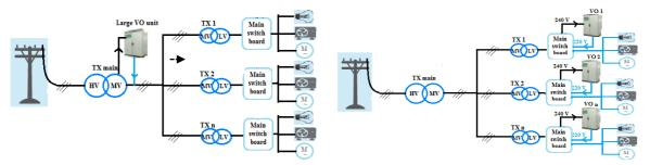
Figure 5: Possible location of VO unit installation in a typical abattoir (a) with main transformer and (b) with individual LV transformer
