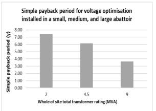
Figure 29: Simple payback period when applying dynamic voltage optimisation with a set voltage of 220V installed at small, medium, and large abattoir with VO units of 2 MVA, 4.5 MVA, and 9 MVA respectively
