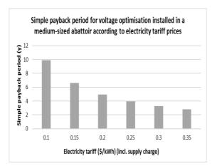
Figure 28: Simple payback period when applying dynamic voltage optimisation with a set voltage of 220V installed at a mediumsized abattoir for a range of electricity tariffs
