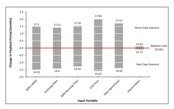
**Figure 3.4: 10% Change in Input Variables - Scenario 6 (500kg/h SGRS) -** Expected change in project payback period when altering individual input variables by ±10%. The baseline case represents project payback period when baseline values for input variables are used, whilst data labels represent project payback period when input variables are altered by ±10%.
