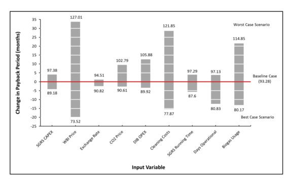
**Extreme Change in Input Variables - Scenario 5 (285kg/h SGRS)** - Expected change in project payback period when individual input variables are altered to possible extreme cases. The baseline case represents project payback period when baseline values for input variables are used, whilst data labels represent project payback period when input variables are altered to extreme cases.
