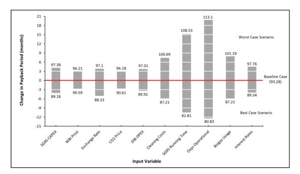
**10% Change in Input Variables - Scenario 5 (285kg/h SGRS)** - Expected change in project payback period when altering individual input variables by ±10%. The baseline case represents project payback period when baseline values for input variables are used, whilst data labels represent project payback period when input variables are altered by ±10%.
