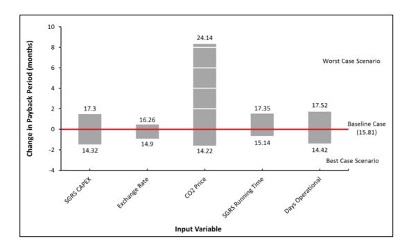
**Figure 3.6: Extreme Change in Input Variables - Scenario 6 (500kg/h SGRS)** - Expected change in project payback period when individual input variables are altered to possible extreme cases. The baseline case represents project payback period when baseline values for input variables are used, whilst data labels represent project payback period when input variables are altered to extreme cases.
