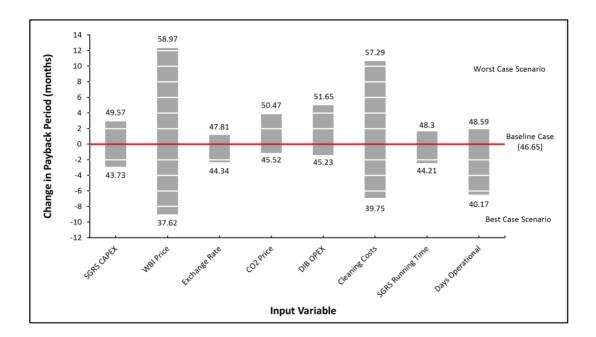
**Extreme Change in Input Variables - Scenario 4 (285kg/h SGRS)** - Expected change in project payback period when individual input variables are altered to possible extreme cases. The baseline case represents project payback period when baseline values for input variables are used, whilst data labels represent project payback period when input variables are altered to extreme cases.
