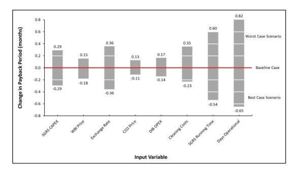
**Focused Sensitivity Analysis - Scenario 4 (285kg/h SGRS)** - Expected change in project payback period when altering individual input variables by ±1% when based on extreme case results. The baseline case represents project payback period when baseline values for input variables are used.
