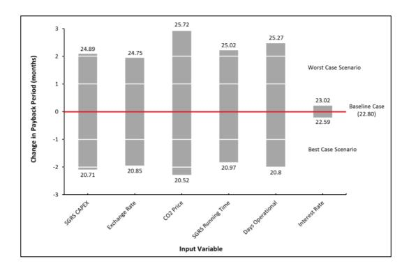
**Figure 3.3: 10% Change in Input Variables - Scenario 6 (285kg/h SGRS)** - Expected change in project payback period when altering individual input variables by ±10%. The baseline case represents project payback period when baseline values for input variables are used, whilst data labels represent project payback period when input variables are altered by ±10%.
