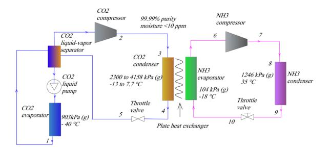
**Figure 2.1: CO<sub>2</sub>-NH<sub>3</sub> Cascade Refrigeration System Design -** Detailed schematic of the closed-loop CO<sub>2</sub>-NH<sub>3</sub> cascade refrigeration system.
