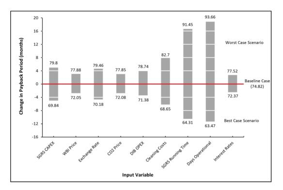
**10% Change in Input Variables - Scenario 3 (285kg/h SGRS)** - Expected change in project payback period when altering individual input variables by ±10%. The baseline case represents project payback period when baseline values for input variables are used, whilst data labels represent project payback period when input variables are altered by ±10%.
