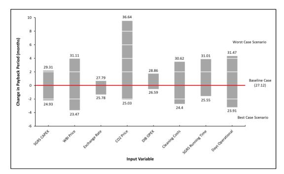
Scenario 3 (500kg/h SGRS) - Expected change in project payback period when individual input variables are altered to possible extreme cases. The baseline case represents project payback period when **baseline** values for input variables are used, whilst data labels represent project payback period when input variables are altered to extreme cases.
