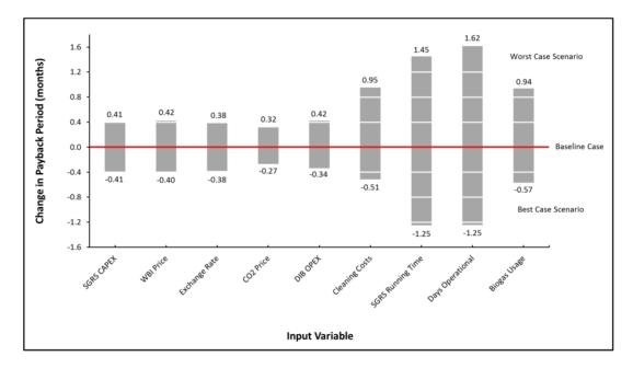
**Focused Sensitivity Analysis - Scenario 5 (285kg/h SGRS)** - Expected change in project payback period when altering individual input variables by ±1% when based on extreme case results. The baseline case represents project payback period when baseline values for input variables are used.
