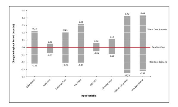
**Focused Sensitivity Analysis - Scenario 3 (500kg/h SGRS)** - Expected change in project payback period when altering individual input variables by ±1% when based on extreme case results. The baseline case represents project payback period when baseline values for input variables are used.
