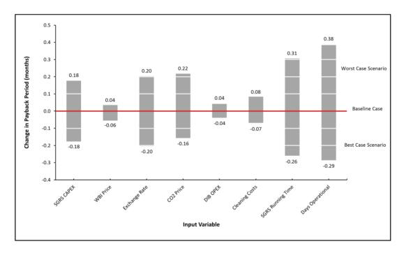
**Focused Sensitivity Analysis - Scenario 4 (500kg/h SGRS)** - Expected change in project payback period when altering individual input variables by ±1% when based on extreme case results. The baseline case represents project payback period when baseline values for input variables are used.
