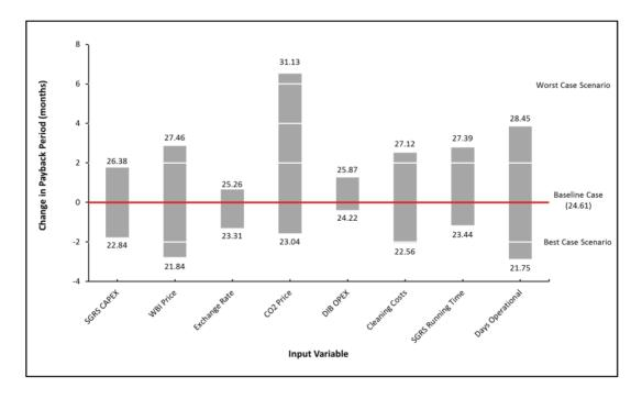
**Extreme Change in Input Variables - Scenario 4 (500kg/h SGRS)** - Expected change in project payback period when individual input variables are altered to possible extreme cases. The baseline case represents project payback period when baseline values for input variables are used, whilst data labels represent project payback period when input variables are altered to extreme cases.
