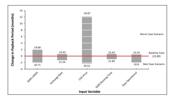
**Figure 3.5: Extreme Change in Input Variables - Scenario 6 (285kg/h SGRS)** - Expected change in project payback period when individual input variables are altered to possible extreme cases. The baseline case represents project payback period when baseline values for input variables are used, whilst data labels represent project payback period when input variables are altered to extreme cases.
