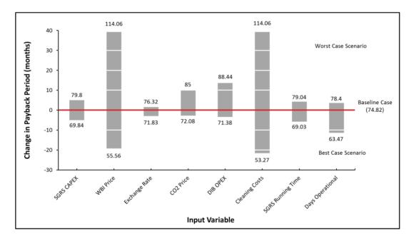
**Extreme Change in Input Variables - Scenario 3 (285kg/h SGRS)** - Expected change in project payback period when individual input variables are altered to possible extreme cases. The baseline case represents project payback period when baseline values for input variables are used, whilst data labels represent project payback period when input variables are altered to extreme cases.
