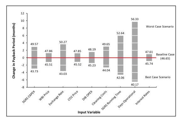
10% Change in Input Variables - **Scenario 4 (285kg/h SGRS)** - Expected change in project payback period when altering individual input variables by ±10%. The baseline case represents project payback period when baseline values for input variables are used, whilst data labels represent project payback period when input variables are altered by ±10%.
