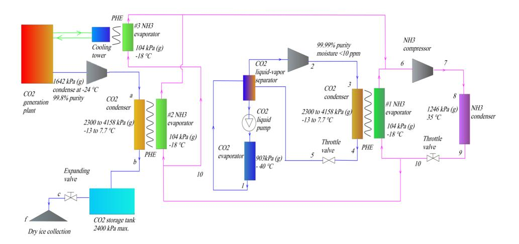
Figure 2.4: Newly Amended System Design - Detailed Schematic of the amended system design of the integrated closed-loop CO<sub>2</sub>-NH<sub>3</sub> refrigeration system and open-loop CO<sub>2</sub> liquefaction system.
