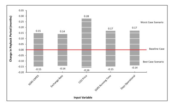
**Figure 3.8:** Focused Sensitivity Analysis - Scenario 6 (500kg/h SGRS) - Expected change in project payback period when altering individual input variables by  $\pm 1\%$  when based on extreme case results. The baseline case represents project payback period when baseline values for input variables are used.
