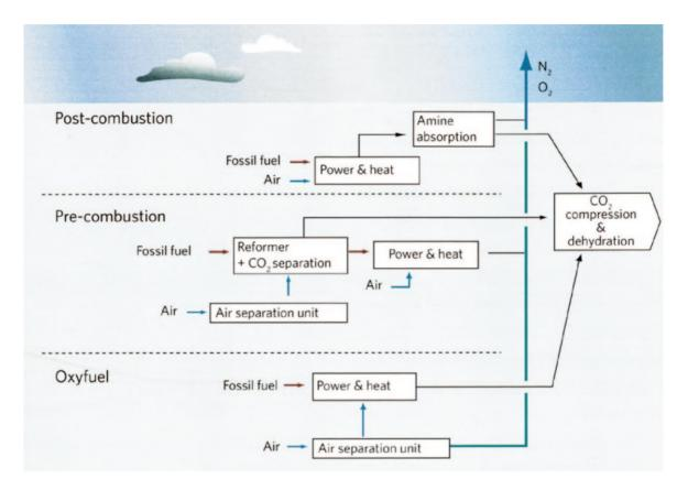
**Figure 2.2: Current CO<sub>2</sub> Capture Methods** - Illustration of the three main methods used for CO<sub>2</sub> capture (Freund & Kaarstad 2007).
