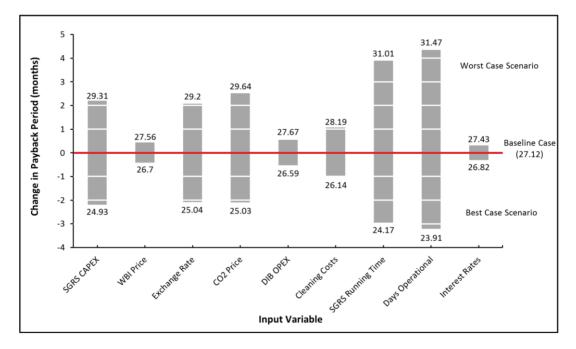
**10% Change in Input Variables - Scenario 3 (500kg/h SGRS)** - Expected change in project payback period when altering individual input variables by ±10%. The baseline case represents project payback period when baseline values for input variables are used, whilst data labels represent project payback period when input variables are altered by ±10%.
