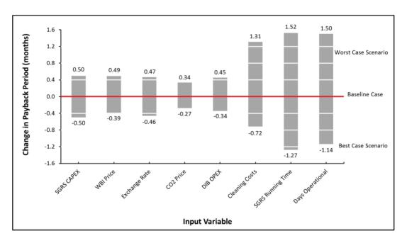
**Focused Sensitivity Analysis - Scenario 3 (285kg/h SGRS)** - Expected change in project payback period when altering individual input variables by ±1% when based on extreme case results. The baseline case represents project payback period when baseline values for input variables are used.
