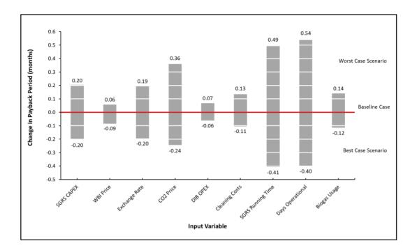
**Focused Sensitivity Analysis - Scenario 5 (500kg/h SGRS)** - Expected change in project payback period when altering individual input variables by ±1% when based on extreme case results. The baseline case represents project payback period when baseline values for input variables are used.
