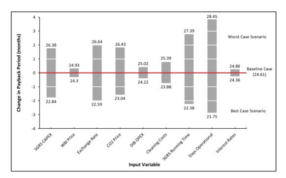
**10% Change in Input Variables - Scenario 4 (500kg/h SGRS)** - Expected change in project payback period when altering individual input variables by ±10%. The baseline case represents project payback period when baseline values for input variables are used, whilst data labels represent project payback period when input variables are altered by ±10%.
