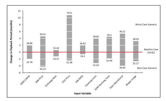
**Extreme Change in Input Variables - Scenario 5 (500kg/h SGRS)** - Expected change in project payback period when individual input variables are altered to possible extreme cases. The baseline case represents project payback period when baseline values for input variables are used, whilst data labels represent project payback period when input variables are altered to extreme cases.
