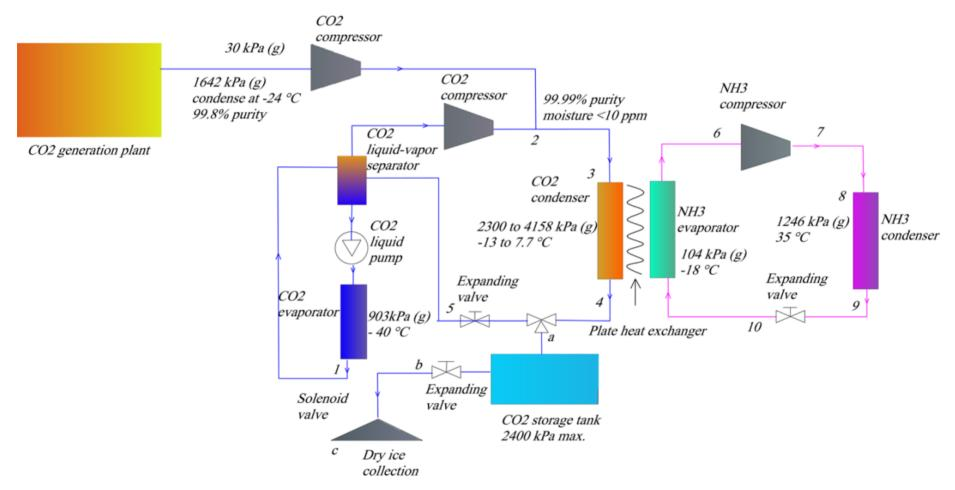
Figure 2.3: Original System Design - Detailed schematic of the integrated closed-loop CO<sub>2</sub>-NH<sub>3</sub> cascade refrigeration system and open-loop CO<sub>2</sub> liquefaction system.
