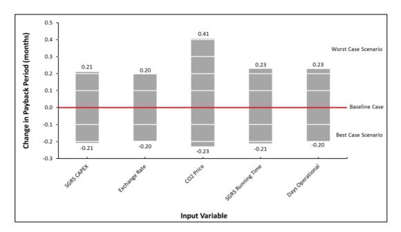
**Figure 3.7: Focused Sensitivity Analysis - Scenario 6 (285kg/h SGRS)** - Expected change in project payback period when altering individual input variables by ±1% when based on extreme case results. The baseline case represents project payback period when baseline values for input variables are used.
