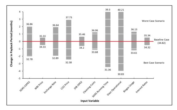
**10% Change in Input Variables - Scenario 5 (500kg/h SGRS)** - Expected change in project payback period when altering individual input variables by ±10%. The baseline case represents project payback period when baseline values for input variables are used, whilst data labels represent project payback period when input variables are altered by ±10%.
