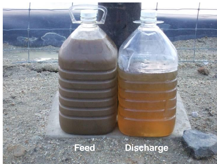
Photo 16: CAL Feed and Discharge
