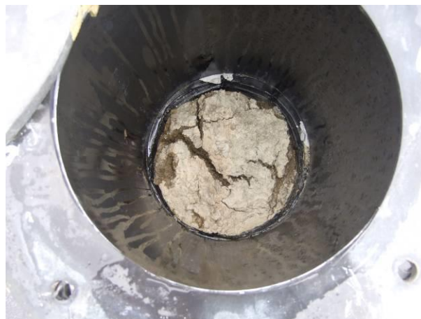
Photo 18: CAL crust at screen end
