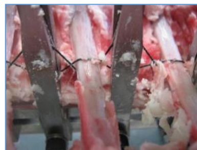
Figure 24: Braid not fully encompassing rib
