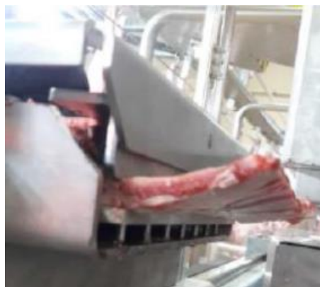
Figure 36: Packing had to be used with the gripper in order to clamp the rack
