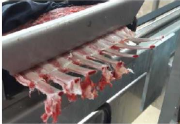
Figure 38: Meat left at the extremity of the bone at the end of the process
