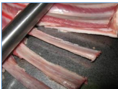
Figure 13: Sinew remained on single scribe removal
