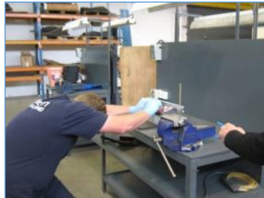
Figure 22: Pulling of Intercostal from Test Rig
