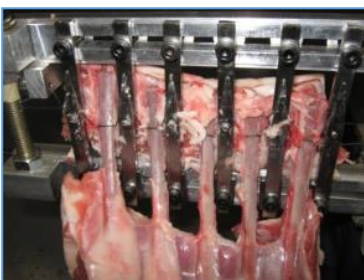
Figure 23 – Intercostal being removed
