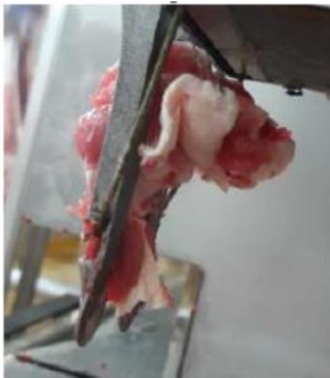
Figure 39: Meat stuck in the top wire, requiring cleaning
