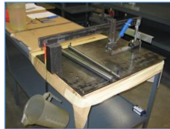
Figure 8: Jug used to apply extra load
