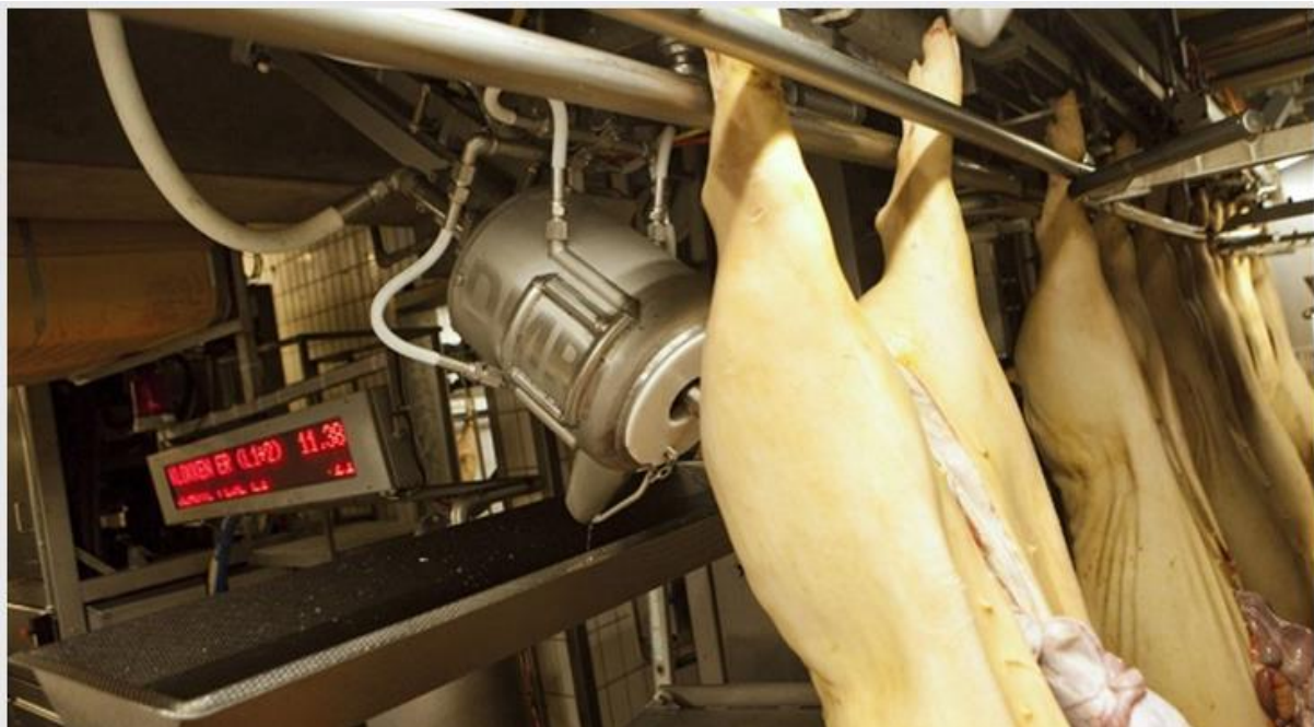
Figure 1. Automatic bung handling equipment in use at a Danish pork slaughterhouse.
