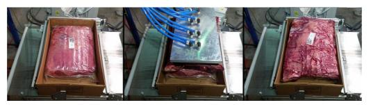
Figure 4: Flat packing process (left to right) for Clod
