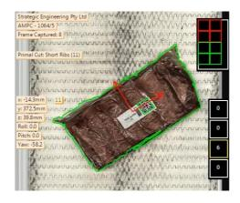
Figure 1: Vision System output detailing pick coordinates and yaw rotation (left), gripper modules to activate (top right), and destination carton and current number of primal cuts in carton (bottom right).
