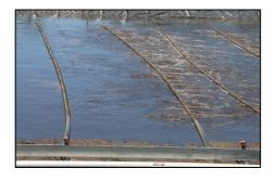
In the Biolac process, the upstream aerated zone provides the nitrate-rich water for the downstream anoxic zone so there is no separate recycle stream. The basin is usually mixed in a manner to minimise the presence of oxygen, for example with submerged mixers. Image: Teys, Beenleigh
