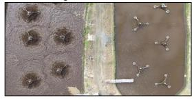
In **Sequence Batch BNR processes**, nitrification and denitrification occur in the same reactor space, but at different times in the cycle. For example, the aeration system turns on for the nitrification part of the cycle, then switches off during the denitrification period. This saves the need for pumping large volumes of liquid around or for separate structures such as clarifiers.
