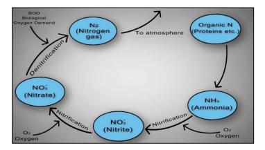
The environment required for each step is radically different. The two technologies provide these two different environments in different ways. Provided the appropriate environment is present, the relevant bacterial will perform the reactions needed to reduce nitrogen levels.
