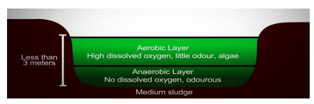
The only difference between a facultative pond and an anaerobic pond is the tonnes of BOD added per unit volume per day. Facultative ponds have a lower BOD added so that the oxygen can penetrate to a reasonable depth before being used for aerobic bacterial activity. The interface between the layers moves up and down according to the amount of aeration of the top layer.
