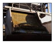
Static screens are usually a vertical bow shaped wedge-wire screen. Most of the liquid drains through the screen while the solids collect at the base before discharge. Image: Meramist, Caboolture
