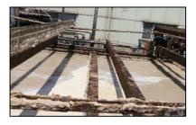
**Dissolved Air Flotation units (DAF)** inject a high-pressure stream of liquid, into the raw wastewater stream which forms a mass of very fine air bubbles that attach to particles and fat globules and lift them to the surface. The floating material is scraped off for disposal or reprocessing and the clean water underneath is discharged.
