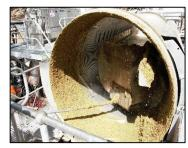
**Rotary screens** use a rotating horizontal cylindrical screen. The solids move to the opposite end of the rotating cylinder, where it discharges. Image: ACC, Cannon Hill
