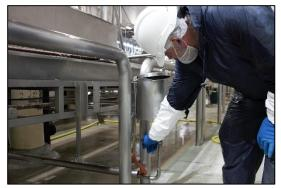
Turning off continuous flow knife steriliser with shut off valve at the end of operations. Image: JBS, Dinmore
