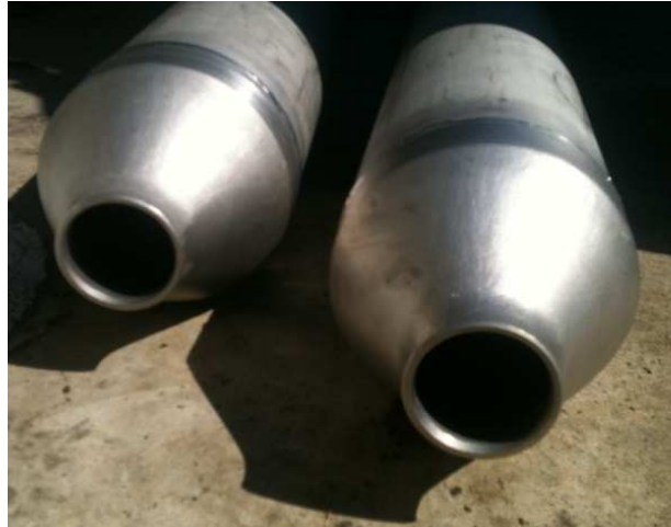
Figure 10: Nozzles used to mix the anaerobic digester pre-installation
