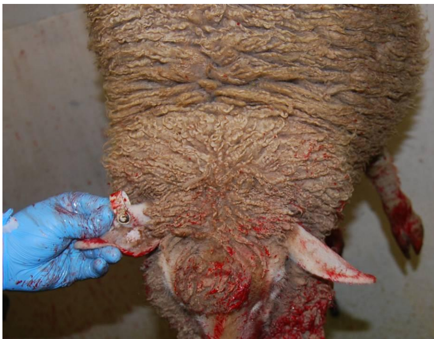
Photo 9-New plastic gambrels can be retro-fitted with RFID tags to carry PIC and other data for the associated carcass.
