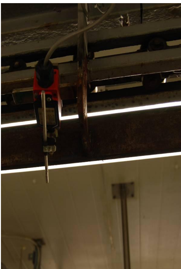
Photos 11 and 11a below – After carcass dressing, the loaded gambrel trips a reader which records that the body number is presenting for disposition; empty gambrel on the right, or “no tag” maintains place in indexing for kill lot.
