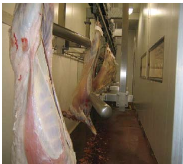
Figure 1. Six-module medium-voltage post-dressing stimulation system. The number of modules (electrodes) is determined by chain speed. With a faster chain, more modules are required to ensure only one carcass is on an electrode at any one time.
