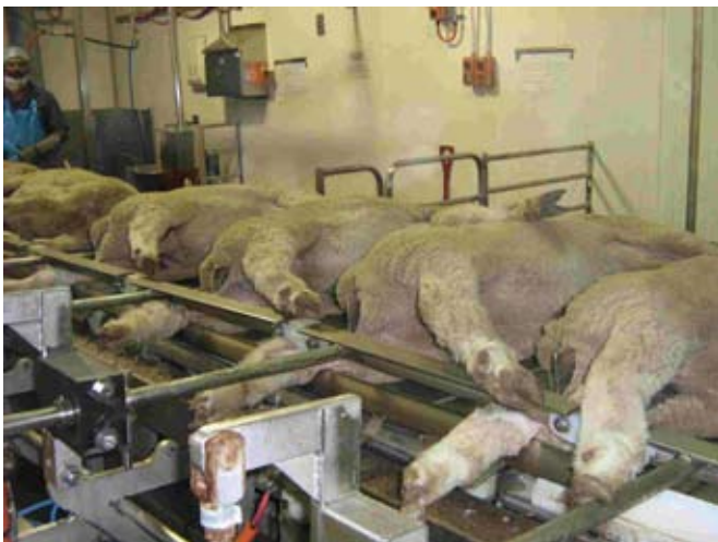
Figure 2. High frequency immobilisation reduces animal movement and permits early and safe commencement of processing.
