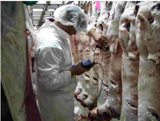
Figure 5. pH and temperature are measured at the lumbar-sacral junction after overlying fat is removed.
