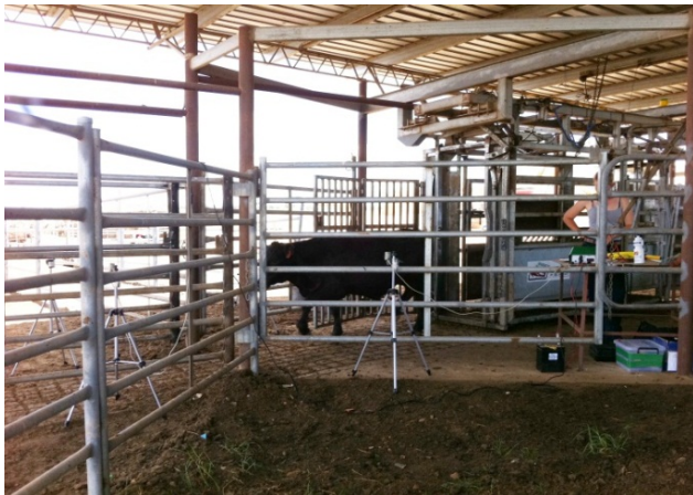
Figure 3- Laser beam apparatus setup for measuring flight speed when animals exit the weighing chute
