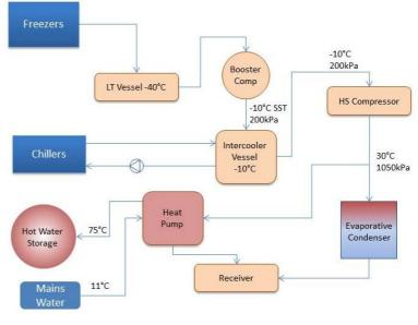
Figure 1 - AHP flow diagram
