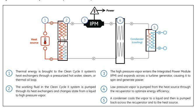
Figure 2: Schematic of commercially available ORC plant<sup>11</sup>
