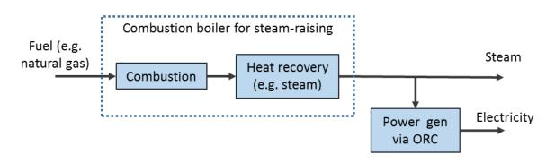
An ORC unit can be incorporated into an existing boiler system. Alternatively it can be installed as part of a boiler upgrade, expansion or replacement.
