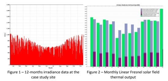
It was found there is an optimal solar field size (aperture area) for all solar thermal technology sited at a given location, with the system sized to meet certain parameters of useful output, for example MegaWatt-hours (MWh) of steam. An aperture area too small will not produce enough thermal output, even at peak solar radiation; an aperture area too large will end up wasting energy and costing too much, despite an seemingly attractive Levelised Cost of Energy.
