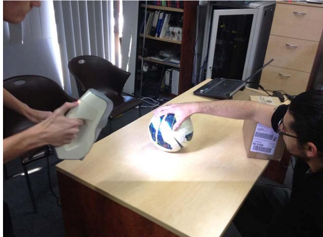
Figure 3 - Using the portable 3D scanning equipment to record a user's hand and arm geometry. Positioning the hand on a ball or similar purpose built jig spreads the fingers to enable a complete scan of the finger geometry and ensures stability during the scanning process (source: WYSIWYG photo)
