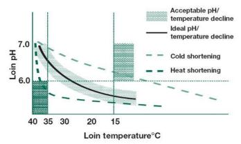
**Figure 1.** pH and temperature decline patterns that can result in heat and cold shortening (Courtesy of MSA).
