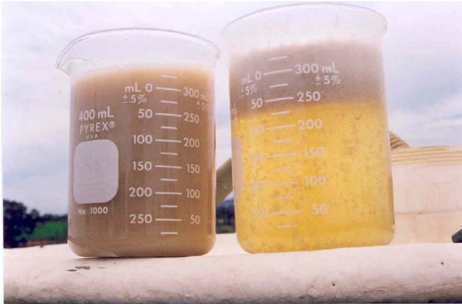
Figure 8: Raw and freshly processed stick water sample
