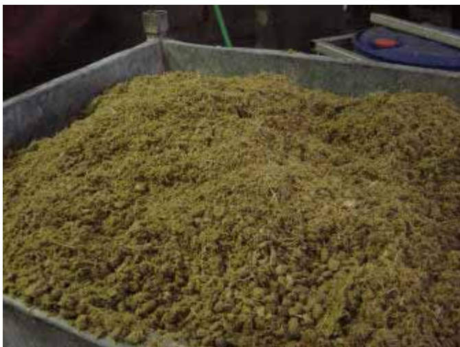
Bin of dewatered paunch solids
