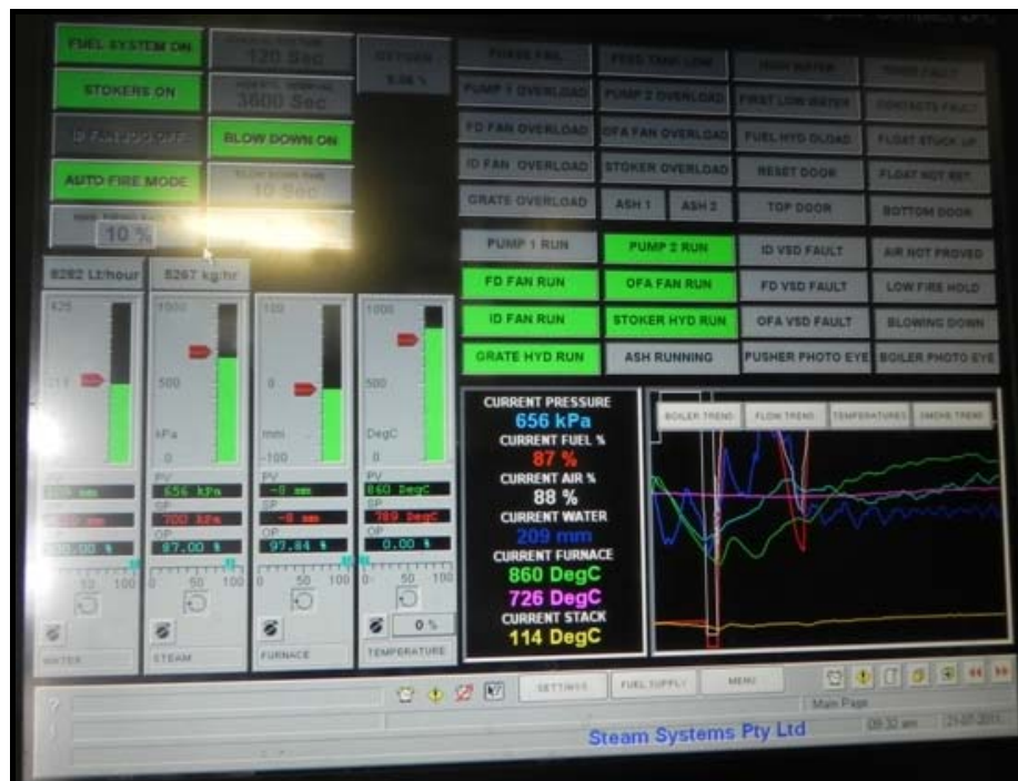
Figure 4.3: Wingham boiler CITECT screen picture
