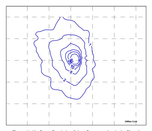
Figure 11.16:  $C_{99 \text{ 1-hr}}$  Rendering Odour Concentration (ou) – Plant 3
