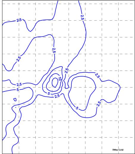
Figure 8.1: C<sub>99.5 1-hr</sub> Odour Concentration (ou) Resulting from 40°C Biofilter Emissions
