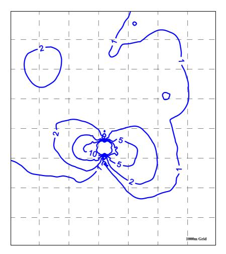
Figure 11.15:  $C_{98 \, 1-hr}$  Rendering Odour Concentration (ou) – Plant 2
