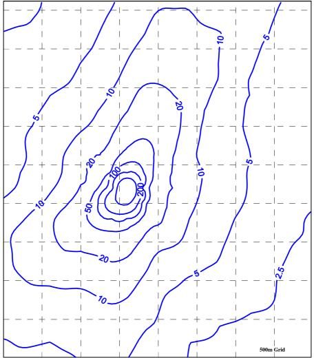
Figure 8.4: C<sub>99.5 1-hr</sub> Odour Concentration (ou) Resulting from 10°C Biofilter Emissions
