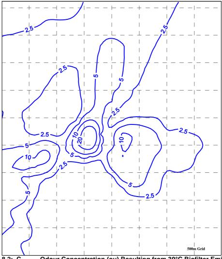
Figure 8.2: C<sub>99.5 1-hr</sub> Odour Concentration (ou) Resulting from 30°C Biofilter Emissions
