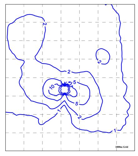
Figure 11.14:  $C_{99 \ 1-hr}$  Rendering Odour Concentration (ou) – Plant 2
