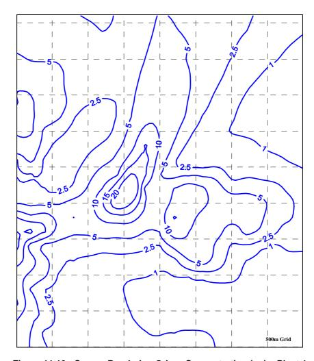
Figure 11.12:  $C_{99.5 \ 1-hr}$  Rendering Odour Concentration (ou) – Plant 1
