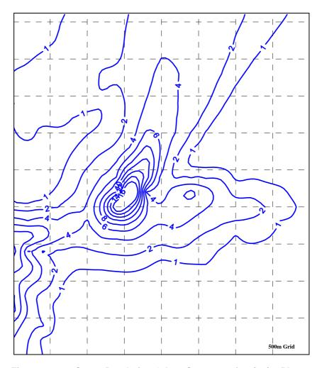
Figure 11.13:  $C_{98 \ 1-hr}$  Rendering Odour Concentration (ou) – Plant 1
