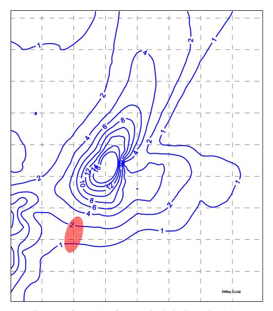
Figure 8.8:  $C_{98\,1-hr}$  Odour Concentration (ou) – Plant 1 Rendering
