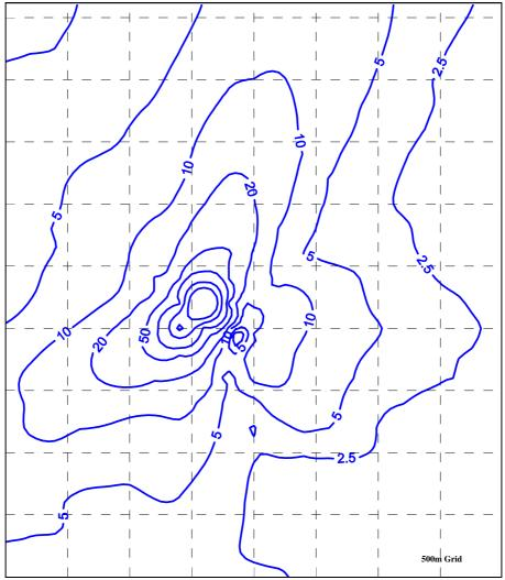
Figure 8.3: C<sub>99.5 1-hr</sub> Odour Concentration (ou) Resulting from 20°C Biofilter Emissions
