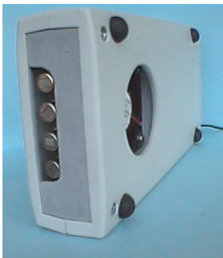
4 sensor array. Dimensions (w x h x d) 100 x 40 x 180 mm Weight (incl batteries) 650 g
