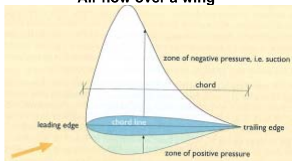
Positive and negative pressure zones created by air flow over a wing 35
