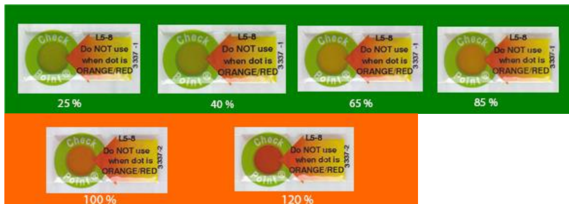
Figure 4. Colour changes of a Vitsab CheckPoint® TTI label ( http://vitsab.com/?page_id=2099 , access on 10 December 2014, with permission)
