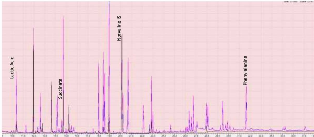
Figure 42: Typical total ion chromatogram profile of saliva and meat methyl chloroformate derivatives. Black trace = saliva blank, pink trace = chew 1, blue trace = chew 10.
