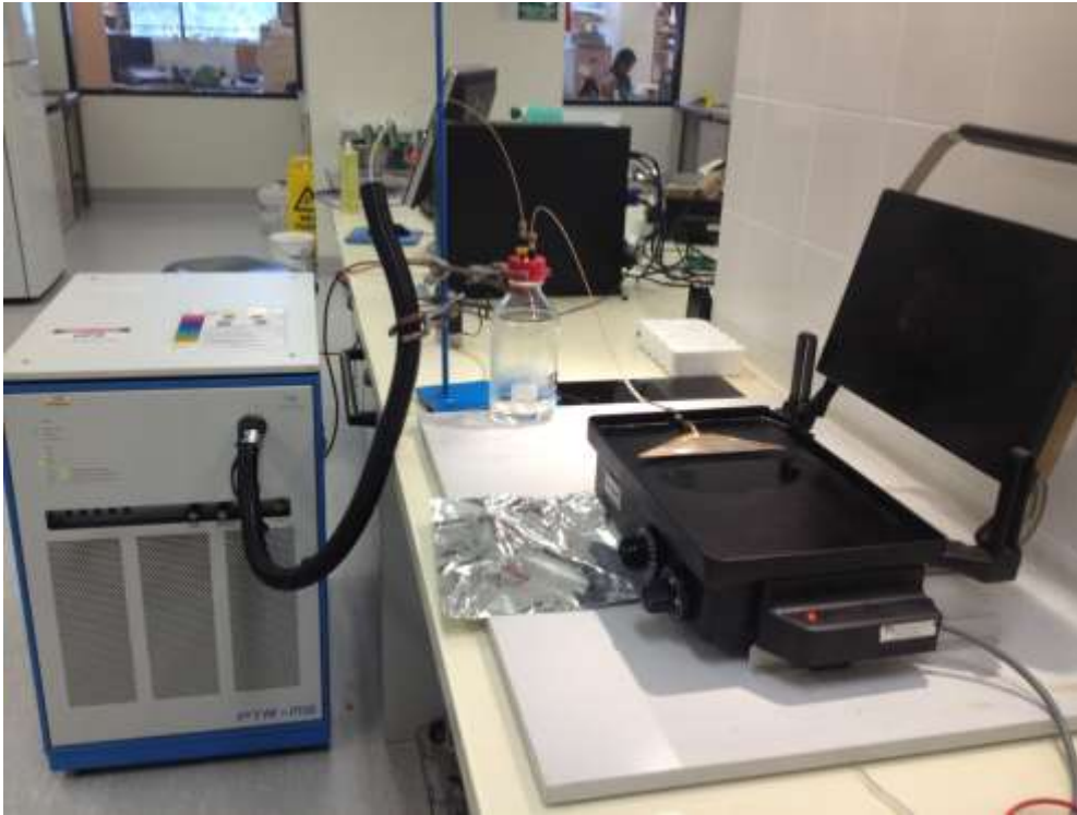
Figure 36: Photograph of the experimental set-up for real time measurement of volatiles during beef grilling. A stainless steel inlet with an opening of 1 mm was attached via a water filter to the PTR-MS inlet.
