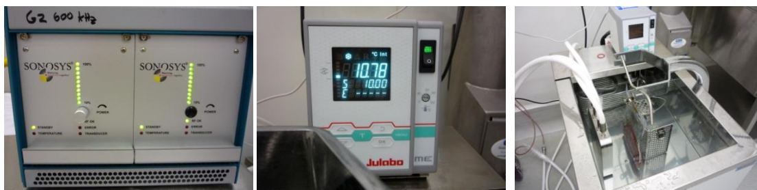
Figure 1: Set-up for ultrasonic trials of post-rigor meat. Left: SONOSYS® generator, Middle: water bath controller, Right: sample immersed in tank, showing position of transducer.
