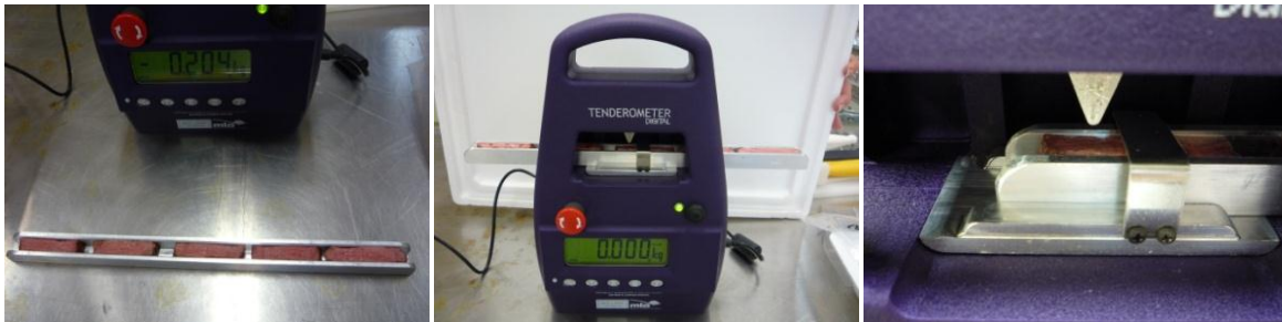
Figure 2: Sample preparation for texture measurement using the G2 Tenderometer. Left, samples placed into texture chamber. Middle, G2 Tenderometer. Right, sample chamber is brought up to the cutting blade.
