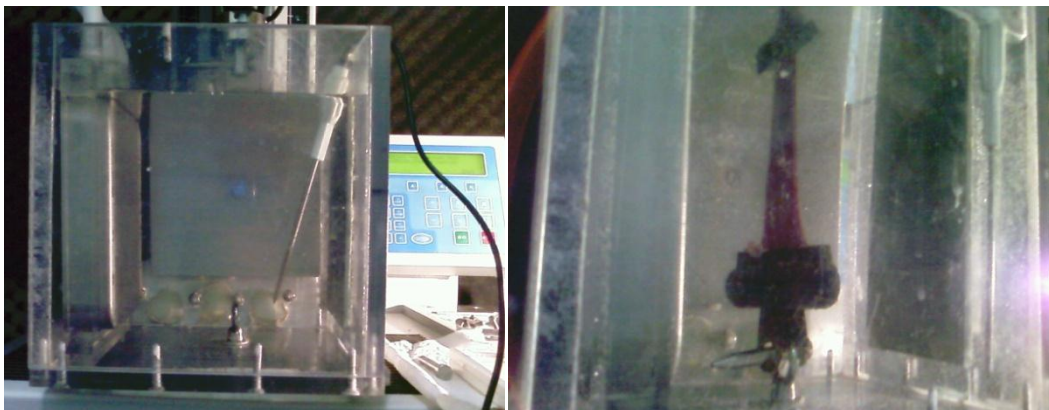
Figure 6: Left, tank and ultrasound setup on Lloyd Universal testing machine platform. Right, sample placement in tank.
